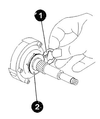
Checking planetary gear train
